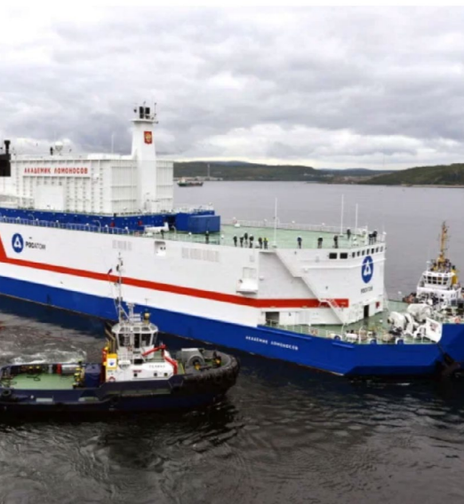
The Akademik Lomonosov is a floating nuclear power plant that holds two nuclear reactors and is stationed in the Chukotka Autonomous area on Russia's Arctic coast.
