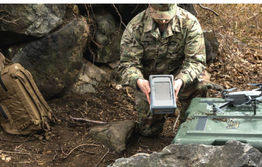
Snowcone is used to run edge computing workloads, or to collect, process, and transfer data to Amazon Web Services.
